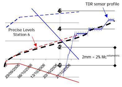
The gradients are very similar (bold black broken line) and the project will be looking at correlations to see if we can 'pattern match' over a season. The slope of the line will of course vary with the soil mineralogy and tree species, height and so forth, although we suspect the profile will be fairly constant as suggested by the work of The Building Research Establishment.
