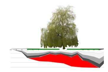
The depth of root activity is exaggerated and we have used precise levels as a proxy for soil testing by increasing the movement profile to coincide with the depth of desiccation for illustration purposes. The soils data reveals the influence of the tree roots extends to around 4mtrs.
