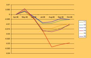
Consistent with the earlier data for the main arrays, we see initial recovery following the winter period and then each of the stations dipping down towards the low point in late August before recovering.
