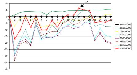
Above we see the results for the end of November. The green line is the high point from May, and the red line is the November reading. We see that at Stations 20 and 21 recovery has already 'lifted' the ground to a point higher than it was in May by nearly 2mm.
